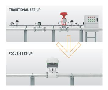
By combining all these components in one device, FOCUS-1 simplifies the installation dramatically and reduces significantly the number of flanges, cables and I/O points.
