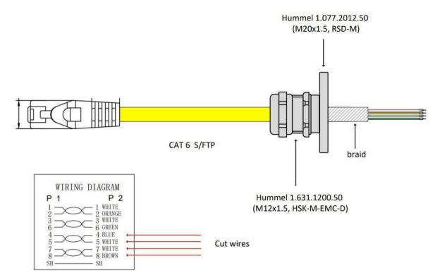
For a stable connection over the ethernet connection, a shielded ethernet cable must be used in combination with the suitable cable gland. Please pay close attention to identifying the right colored cables and connector numbers, and use cable lugs for a robust connection.
