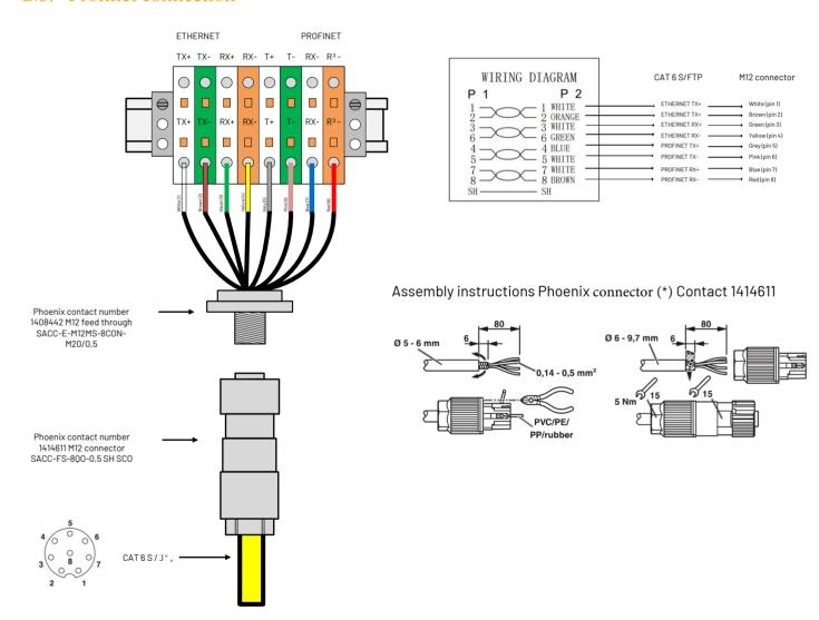
For further detail about the Profinet connection the device to a PROFINET IO network, consult FOCUS-1 Profinet Supplementary Instructions (TD-088) and Assembly instruction (TD-091).
